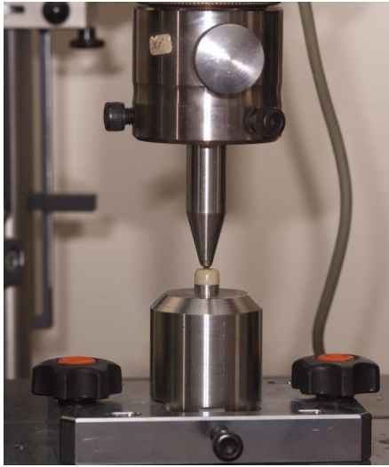
Figure 3. Universal testing machine showing fracture resistance test
