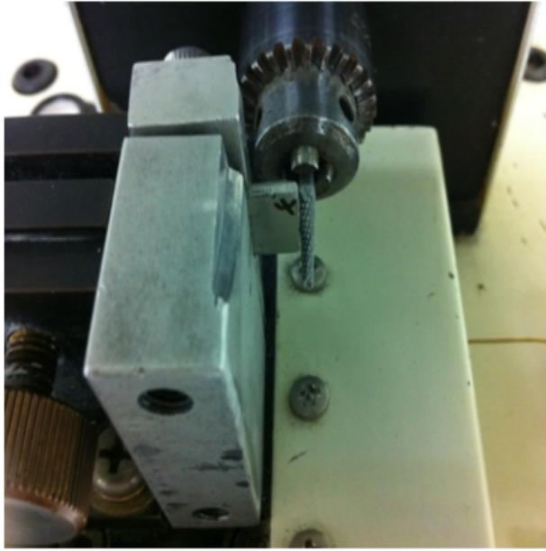
Figure 1. The photo of grinding tester for measuring machinability.
