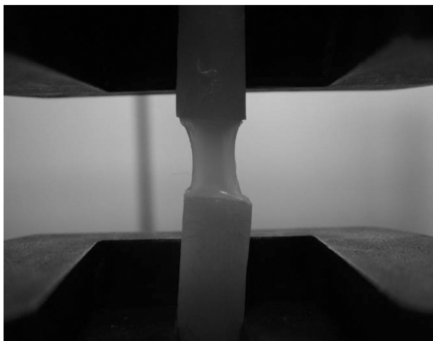
Figure 1. Tensile test specimens in universal testing machine.
