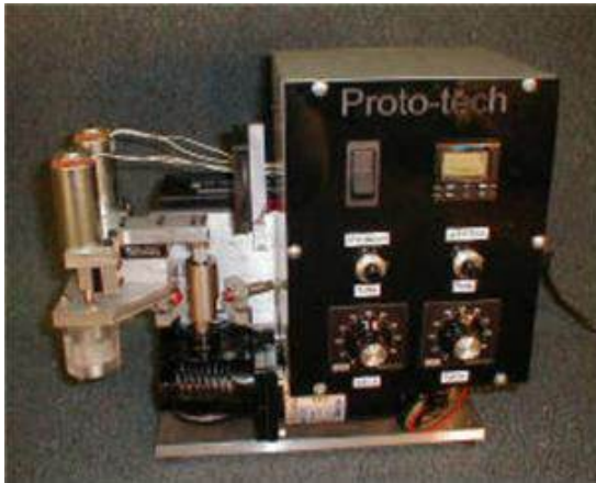
Figure 1, OHSU oral wear simulator.
