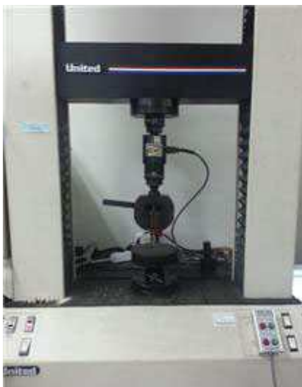
Figure 2. Schematic diagram of the compression test set-up on UTM.
