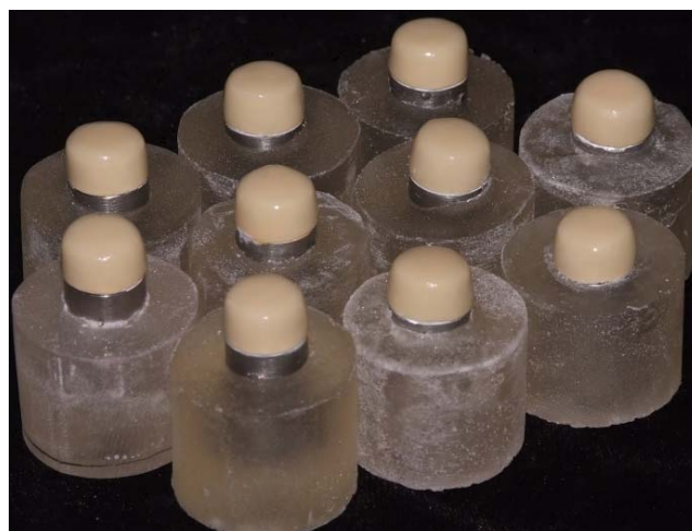
Figure 3. Completed specimens seated on metal master dies that were impregnated in acrylic resin.
