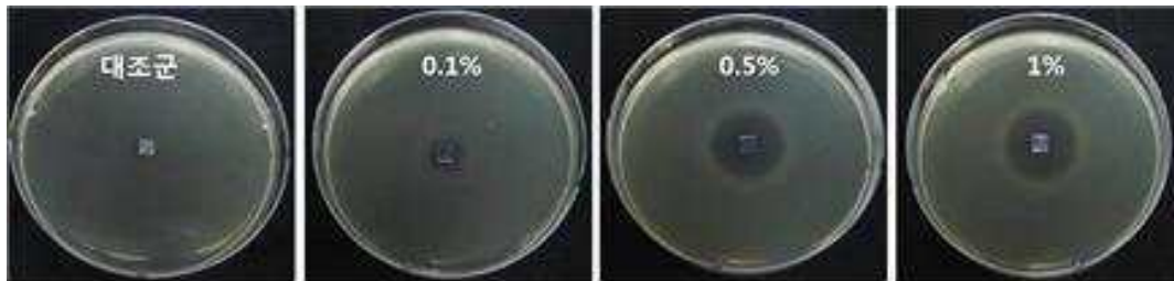
Figure 4. Antibacterial effects by Agar diffusion test of control vs. gold nanorods(GNRs) coated titania nanotubes with the concentration of tetracycline.
