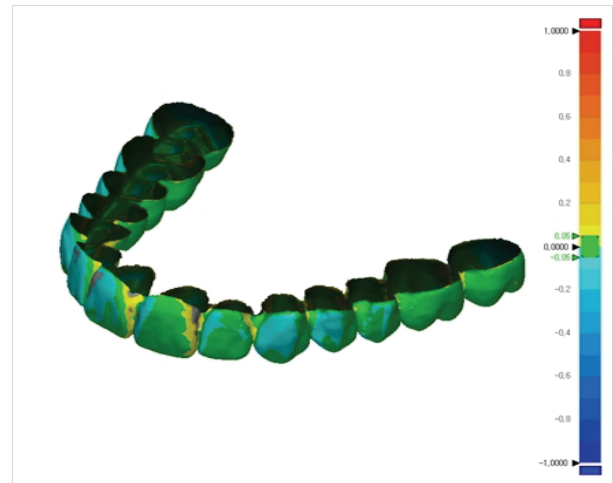
Figure 3. Color map showing volumetric difference between the scanned images of original model and 3D printed model.
