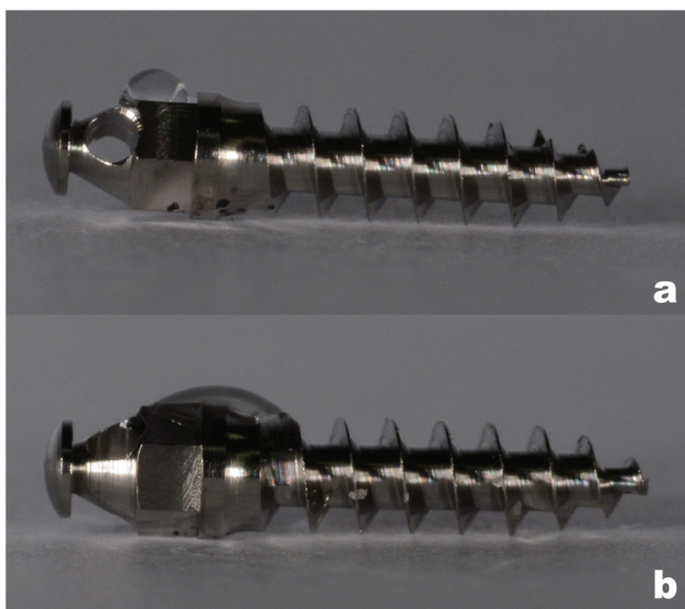
Figure 2. Water contact angle test results conducted on the newly manufactured microimplants; a: Autoclaved microimplants, b: Autoclaved + UV treated samples,
