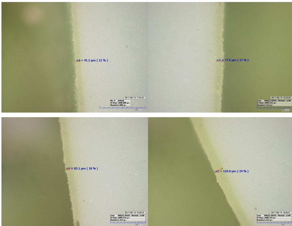
Figure 3. Measurement of Silicone replica film thickness using digital microscope ( \times 140 )
