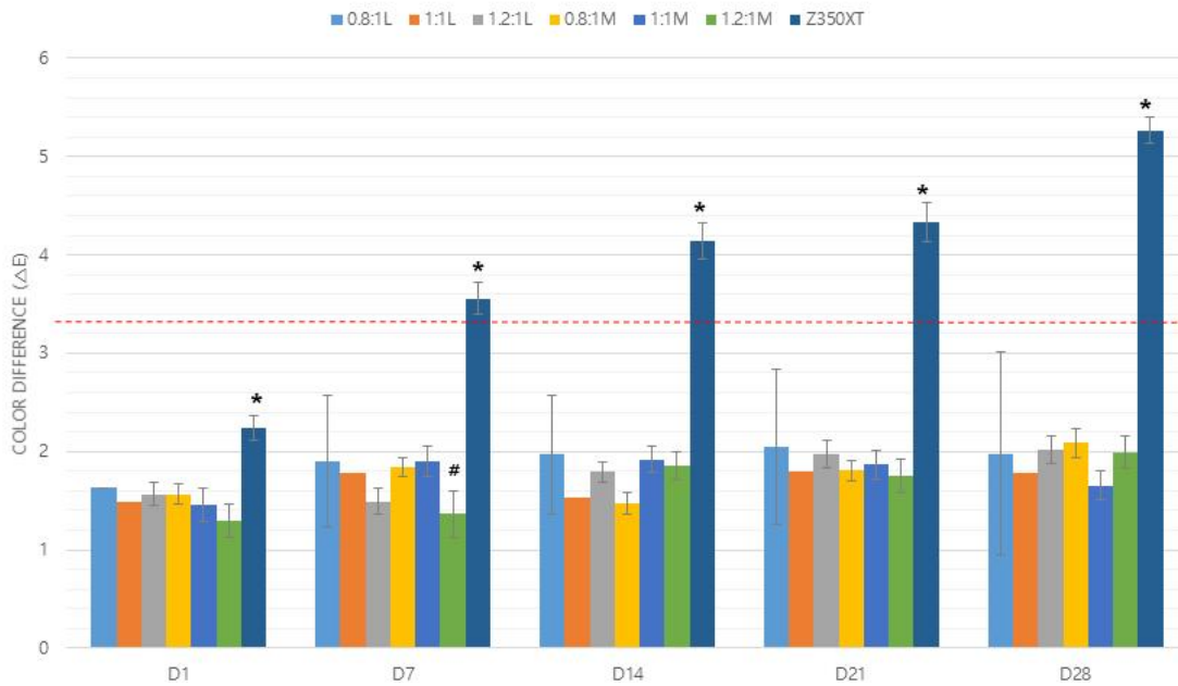
Figure 1. \Delta E values for all of the groups at the different measurement time. The values of \Delta E > 3,3 are considered as clinically unacceptable color difference. *,# Indicate the significant differences among all groups ( p < 0,05 ).
