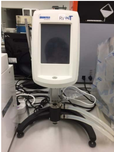
Figure 2. Viscometer to measure the viscosity of resin tested in the experiment.
