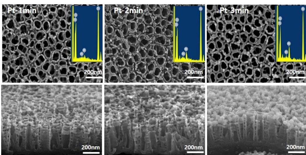
**Figure 3.** FE-SEM micrographs ( $\times 100,000$ ) top view & Cross-sectional view of Pt-TiO<sub>2</sub> NTs; Inserted top right images display the surface elements of Pt-TiO<sub>2</sub> NTs by EDX.
