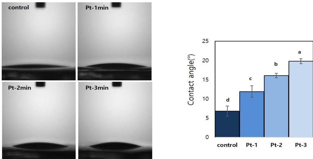
**Figure 4.** Surface contact angles and water drop profiles of the  $\text{TiO}_2$  NTs and Pt- $\text{TiO}_2$  NTs; Schematic of the water contact angle for the four groups:  $\text{TiO}_2$  (control), 1 min coated Pt- $\text{TiO}_2$  NTs, 2 min coated Pt- $\text{TiO}_2$  NTs, 3 min coated Pt- $\text{TiO}_2$  NTs. Different lowercase letters are significantly different ( $P<0.05$ ).
