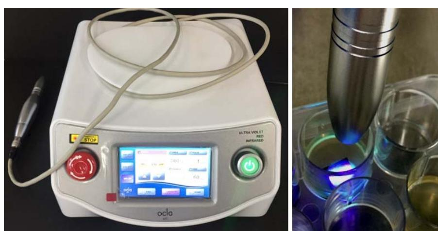
**Figure 1.** Passive cooled InGaAs diode laser and Image of 405 nm laser irradiation on Pt-TiO<sub>2</sub> Nanotubes.
