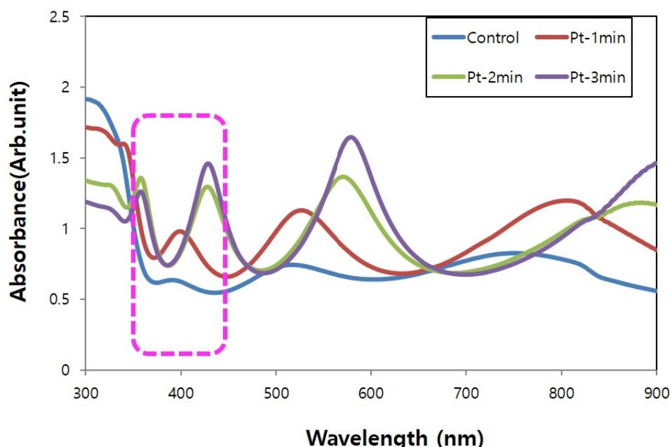
**Figure 2.** UV-vis diffuse reflectance absorption spectra of Pt-TiO<sub>2</sub> NTs; Diffuse reflectance UV-Vis–NIR spectrophotometry dotted line indicated the light absorbance range of 1min coated Pt-TiO<sub>2</sub> NTs was only suitable for 405 nm laser irradiation.
