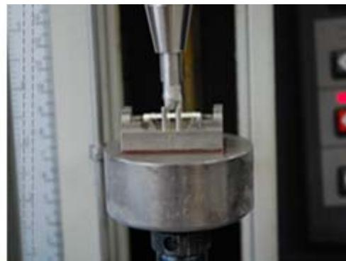
**Figure 2.** Experimental setup (a) and three-point flexural test (b).
