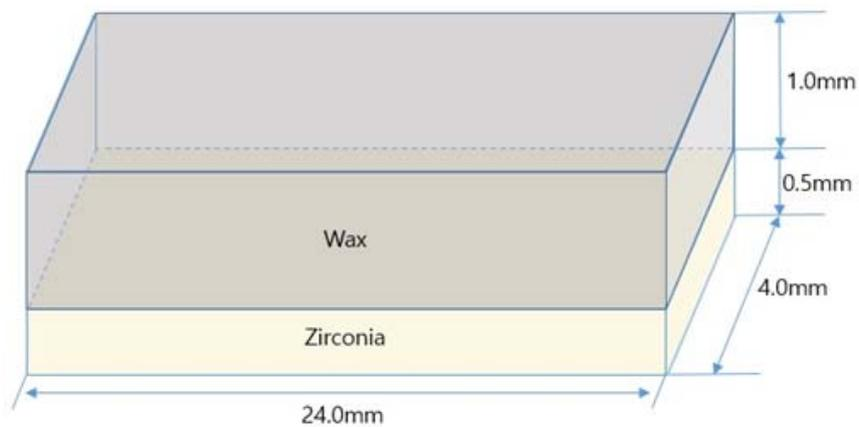
**Figure 1.** Schematic diagram of specimen.
