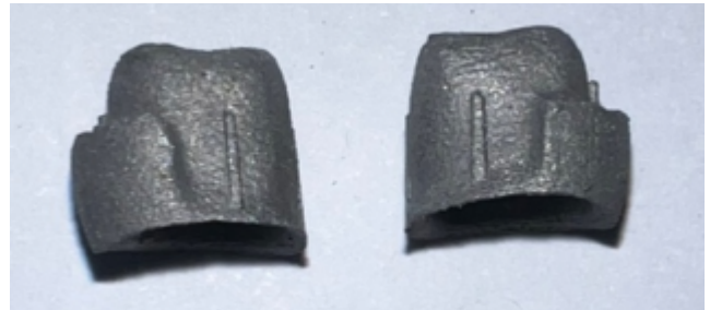
Figure 2. Polished Co-Cr alloy coping after SLS printing.
